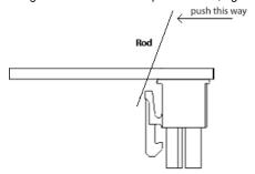
Fig 1.0, releasing the connector latch
